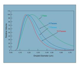
Above: The effect of up to 10 discrete passes at 1000 bar on an oil-in-water intravenous emulsion. Each pass results in a shift of the particle size distribution towards smaller droplet sizes.
